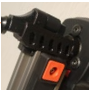
Keyless Jam Clearing
